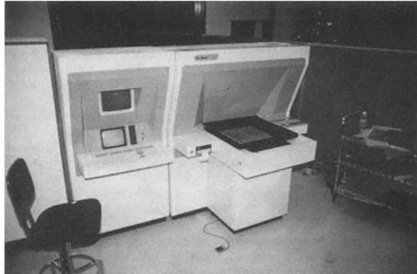
Figure 2.6 Early version of an Orbot (now part of Orbotech) printed circuit board trace inspection system.
