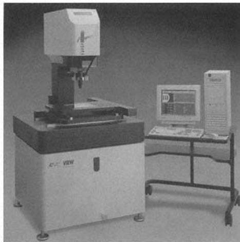
Figure 2.5 Version of an off-line dimensional measuring system "Voyager" offered by GSI Lumonics.
