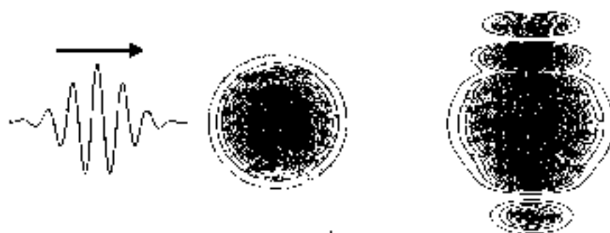
Fig. 1.4 Schematic illustration of density fluctuations, deformations, and ionization of an atom hit by an intense laser pulse. The right figure is a snapshot of the highly excited atom, which emits packets of electronic density into the continuum. Processes such as this typically take place within a few tens of femtoseconds.
