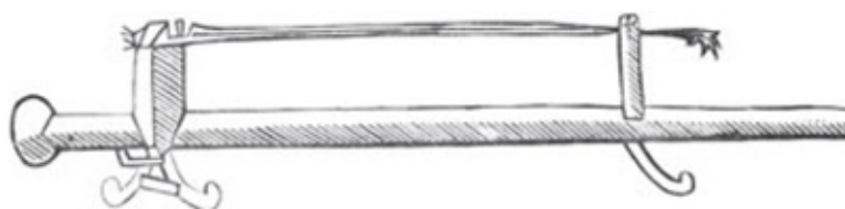
Dame Juliana includes an illustration of a device for making horsehair lines.
