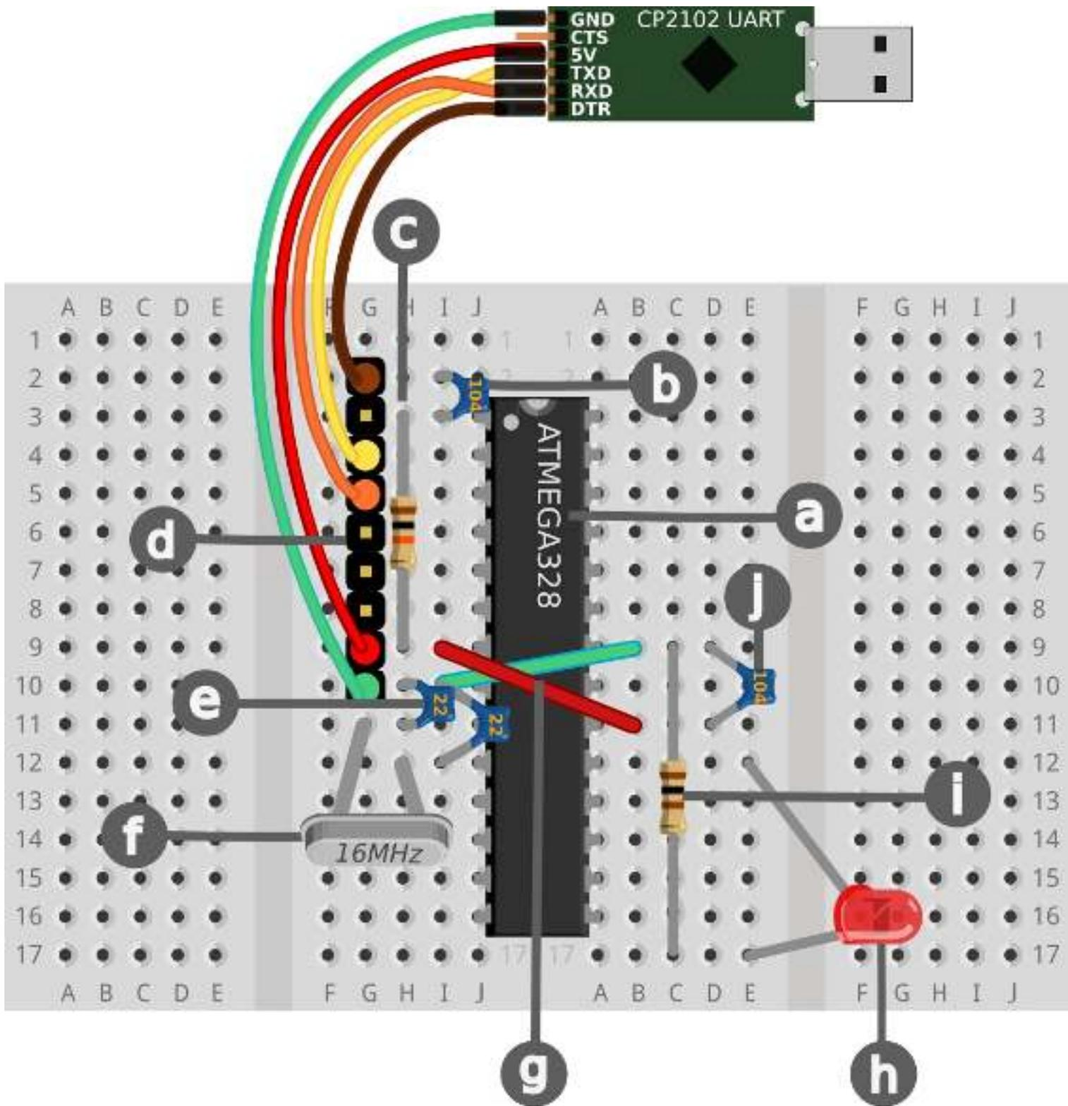
Figure 2-5. The complete DIY microcontroller circuit
