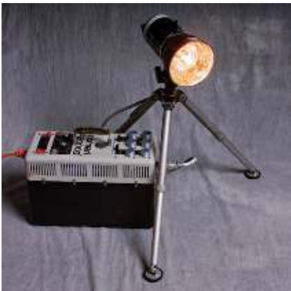
TOP LEFT—This is a Norman LH2400 head and a 2000 watt-second pack. While this gear is a little heavier than monolights, it can still be useful if you need a lot of power (e.g., if you are lighting a building from the outdoors at night). TOP RIGHT—I shot this bar with quartz lights so I could integrate a little more of the existing room light. BOTTOM RIGHT—This is a Smith-Victor quartz light. I have some of these that I have used for decades. They can extend your reach because you can use long exposures with them. A 30-second shot with a quartz light can give you a lot of light.
