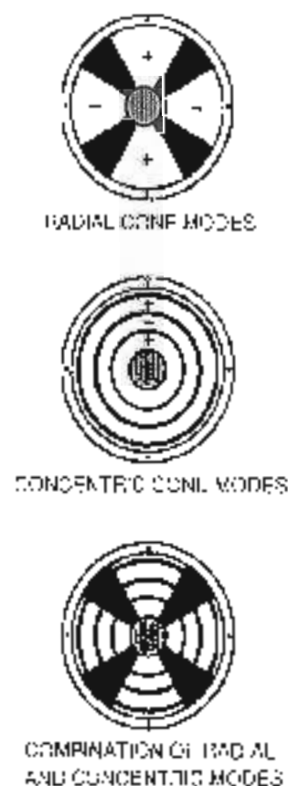
FIGURE 6.19: Cone vibration modes.
