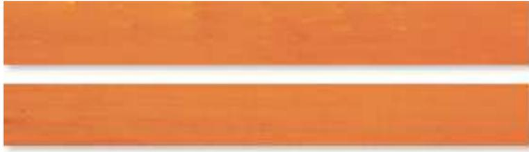
Redwood was the original decking material, chosen for its incredible color and enthralling grain patterns. There are 30 different grades of redwood but only a handful are used for decks. The better the grade, the fewer visible imperfections such as knots, and the more resistant the wood will be to insect and moisture-related problems. Look for clear all heart (shown above), clear, or clear heart grades, to construct a high-quality, lasting deck.
