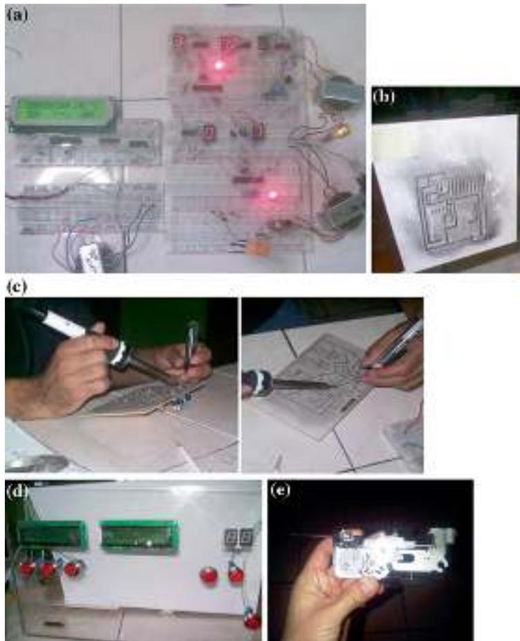
**Fig. 4** Electronic design and analysis of shape memory material: (a) the temperature controller circuit, (b) printed circuit board, (c) solder components, (d) full box (Push button, indicators, LCD displays, switch and connection to electrodes) and (e) terminals and box components (terminal stripping of liver tumors: shortest amount of time and high accuracy to improve security of the process)
