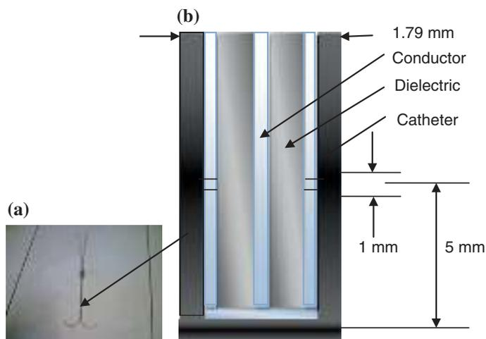
**Fig. 2** Antenna geometry for microwave coagulation therapy. **a** A coaxial cable with a ring-shaped slot cut in the outer conductor which produces a short circuit at the tip. **b** A plastic catheter surrounding the antenna
